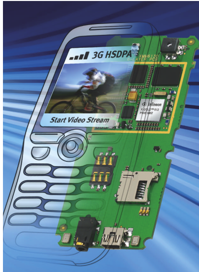
The XMM 6130 platform targets the entry-level Internet-browsing-phone market, supporting 3G HSDPA. It integrates an ARM11-based microcontroller, baseband digital and analog features, and power-management functions (courtesy Infineon).
